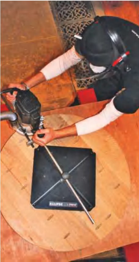
▲ Pic.14 Routing the perfect circle using Trend's ellipse and circle cutting jig
